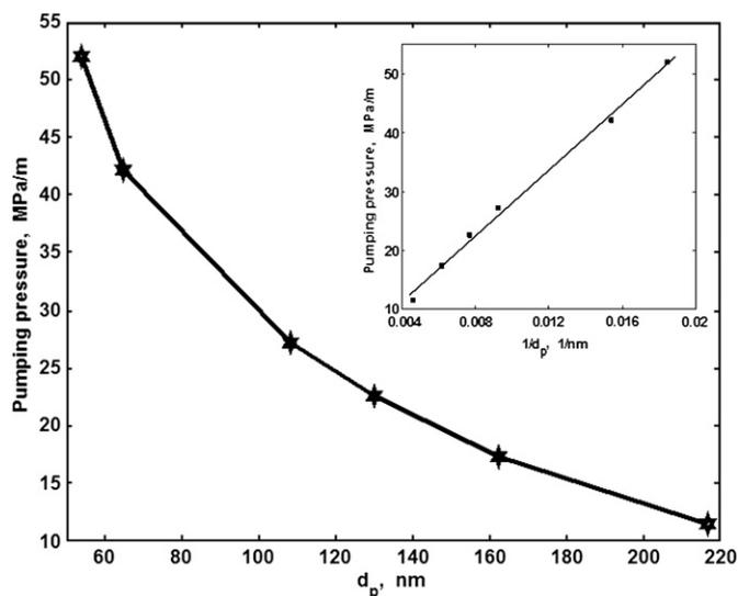
Fig. 4. Maximum pumping pressure vs particle diameter.
