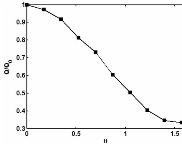
Figure 6: The flow rate versus the orientation angle  $\theta$  when  $a=61.5$  nm and  $b=40.6$  nm. The flow rates are normalized by the case when  $\theta=0$ .
