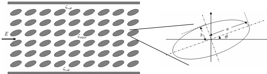
Figure 3: Schematic illustrations of the ellipse array packed in a microchannel and the microstructure of each ellipse.
