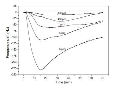
However, the fiber QCM sensors could not detect low concentrations of ammonia gas at very low relative humidity. Therefore, the pre-sorbed moisture in fibrous membranes was proven to be the key
