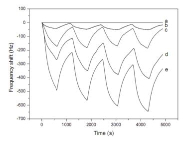
The results of sensing experiments indicated that the sensitivity of the fibrous PAA membranecoated QCM sensors was four times higher than that of the casted PAA film-coated QCM sensors. Moreover, the fiber-coated QCM sensors with small average fiber diameters had higher sensitivity towards low concentrations of ammonia, as low as 130 ppb at a relative humidity of 40 % (Figure 4).
