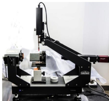
Fig. 3. Contact angles of sliding drops on vertical walls under gravity. The experiments were performed on DSA25, KRÜSS in (a). The moving drop shape under a steady state from our experiments is shown in (b). (c) Shows the result from our simulations. In the experiments, deionized water drops slid under gravity on a vertical plastic wall. The white dashed line in (b) is a reference line of the drop bottom.
