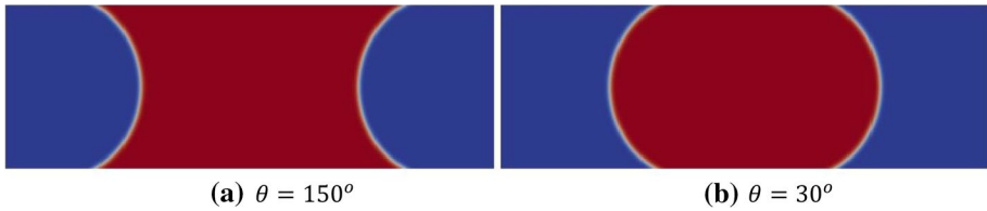
Fig. 4 Equilibrium distribution of fluid column in capillary tube for a \theta = 150^\circ and b \theta = 30^\circ
